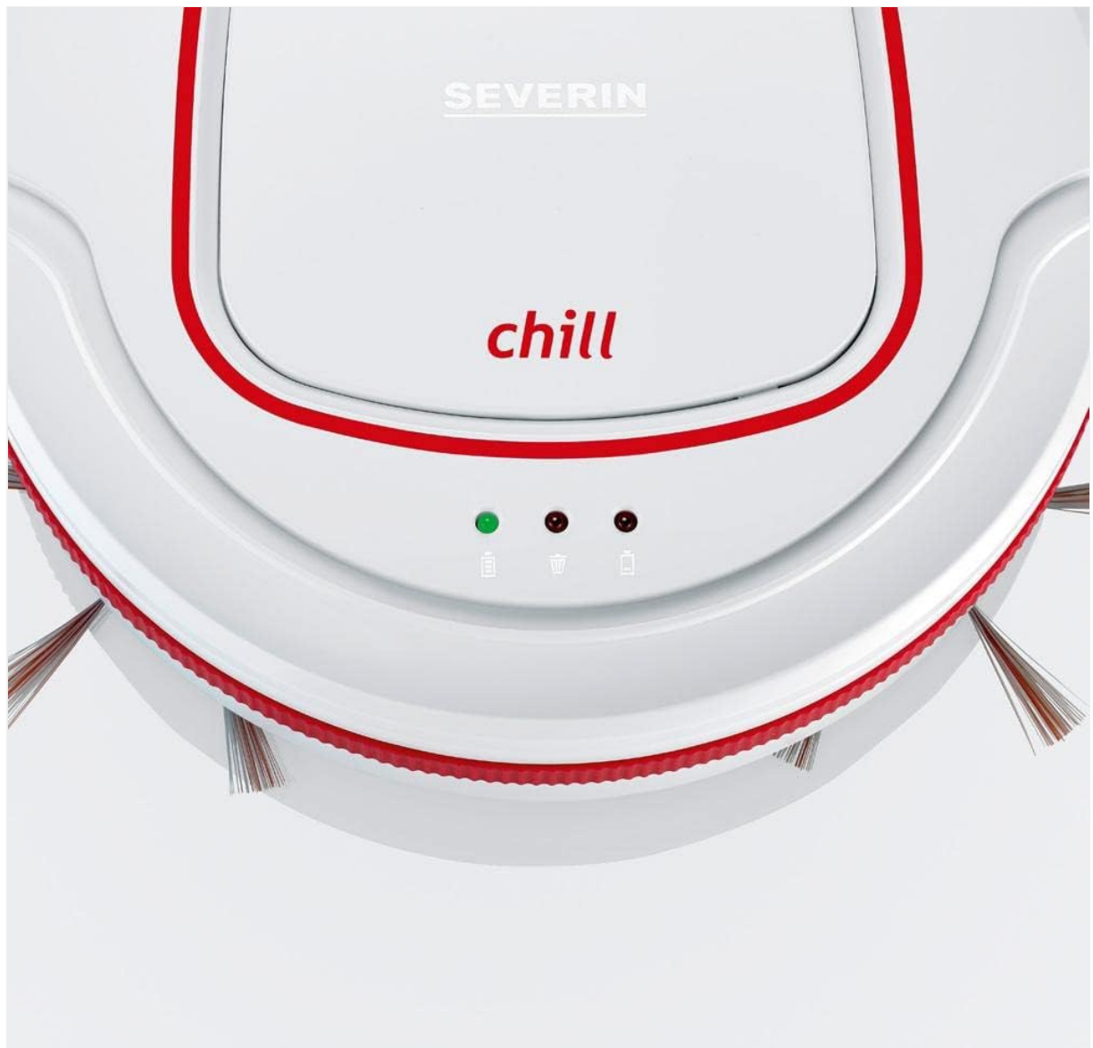
Figure 3.2: Detail of the indicator lights and dustbin icon on the robot's top panel, indicating status and dustbin full.
