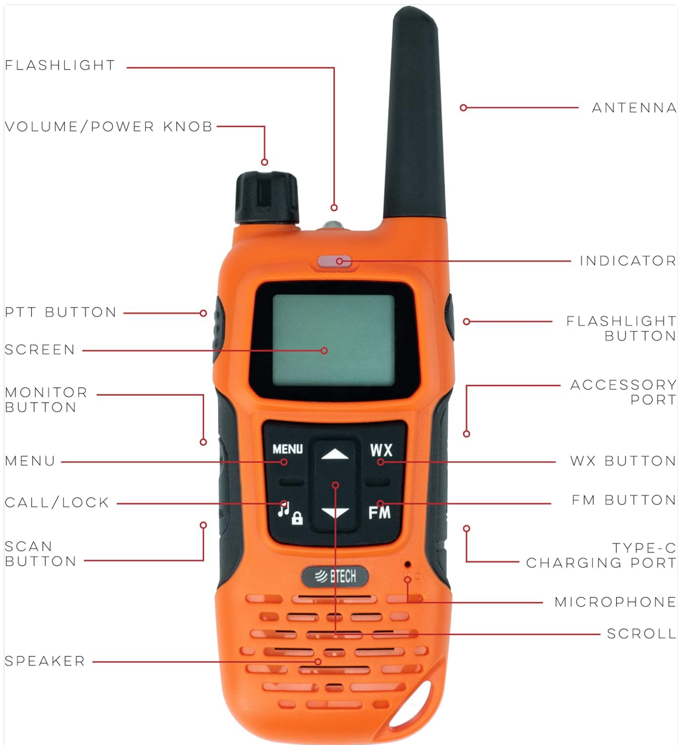
Figure 2: FRS-A1 Radio Components
