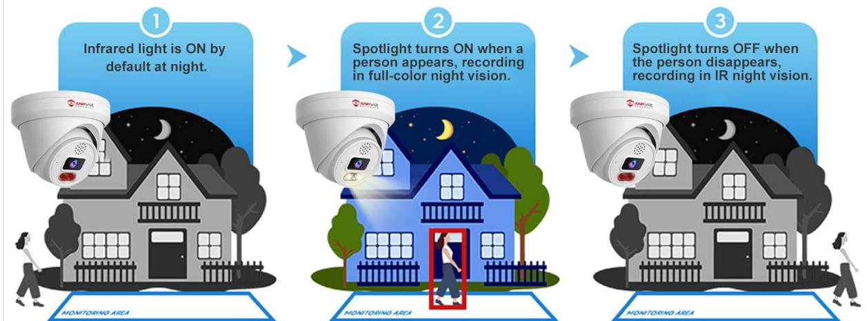
Figure 7: Diagram explaining the Smart Dual Light Color Night Vision modes.
