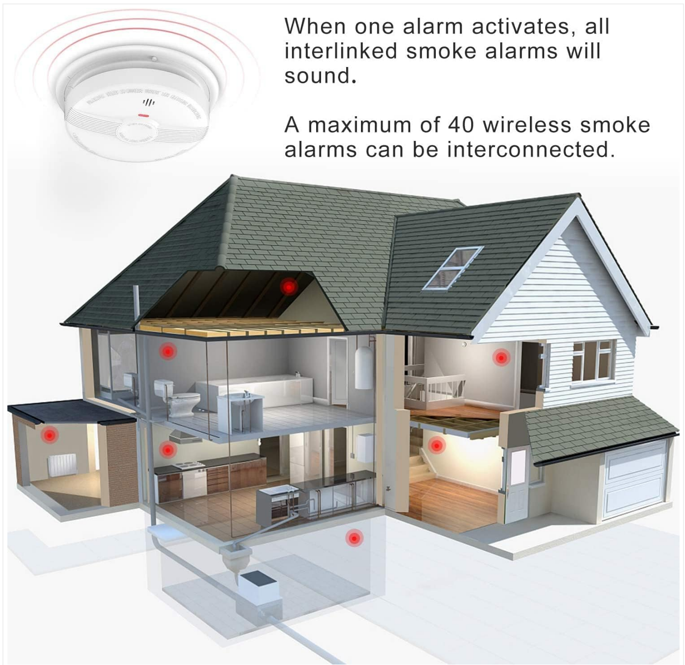
Image 4.1: Recommended smoke detector placement throughout a typical home. When one alarm activates, all interlinked smoke alarms will sound. A maximum of 40 wireless smoke alarms can be interconnected.
