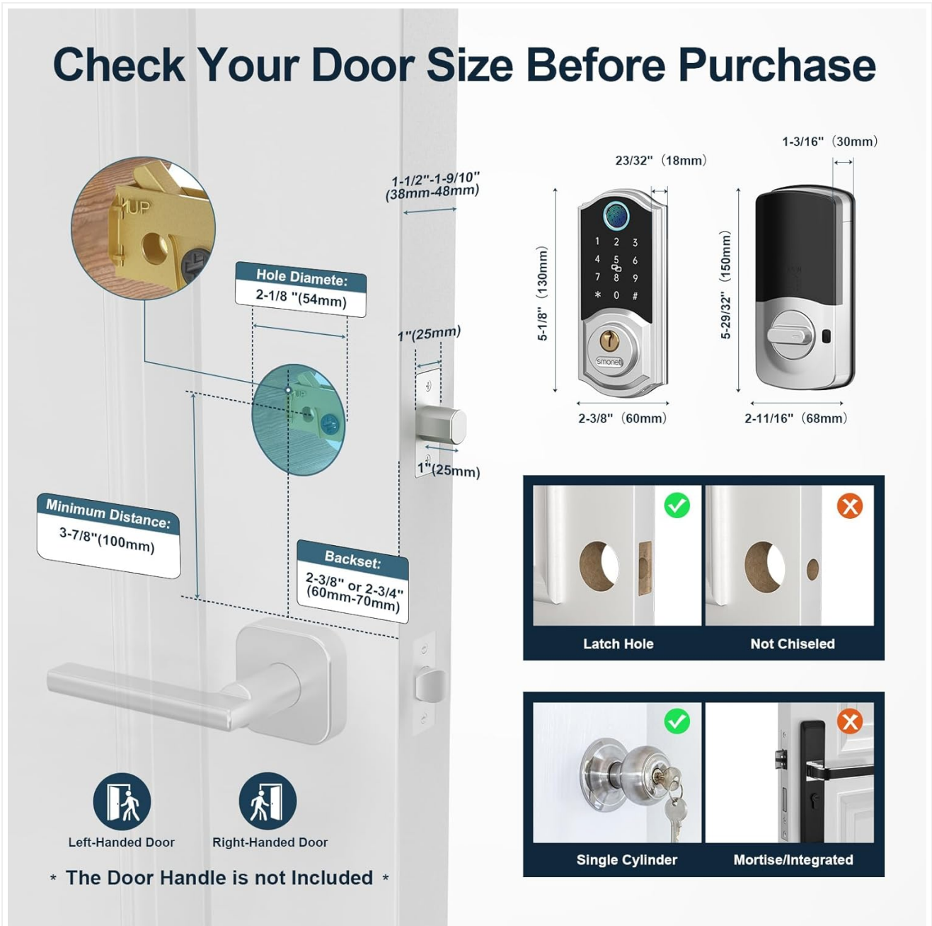
Image 4.1: Door measurement guide and compatibility checks for the SMONET Smart Deadbolt.
