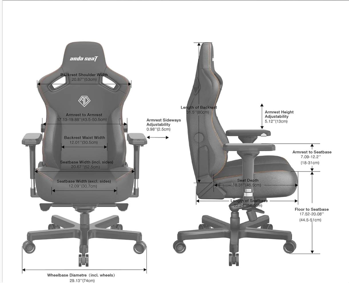
Image 8.1: Technical drawing displaying all key dimensions of the Anda Seat Kaiser 3 chair, including seat width, backrest height, and armrest adjustability.
