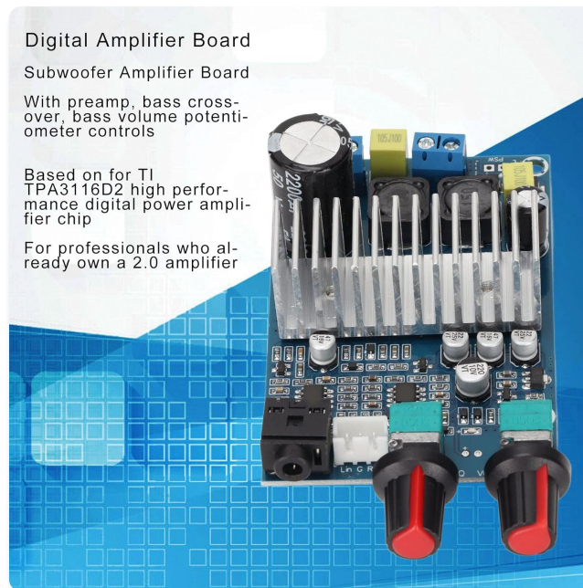
Image: The amplifier board with text overlays indicating its preamplifier, bass crossover, and volume potentiometer controls, and its high-performance digital amplifier chip.
