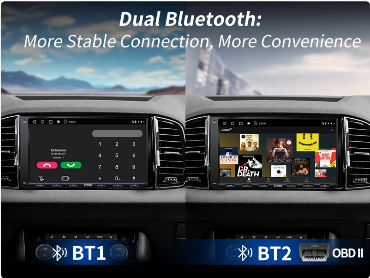
Figure 5.11: Demonstrates the dual Bluetooth capabilities, allowing for simultaneous phone calls/audio streaming (BT1) and connection to other Bluetooth devices (BT2).
