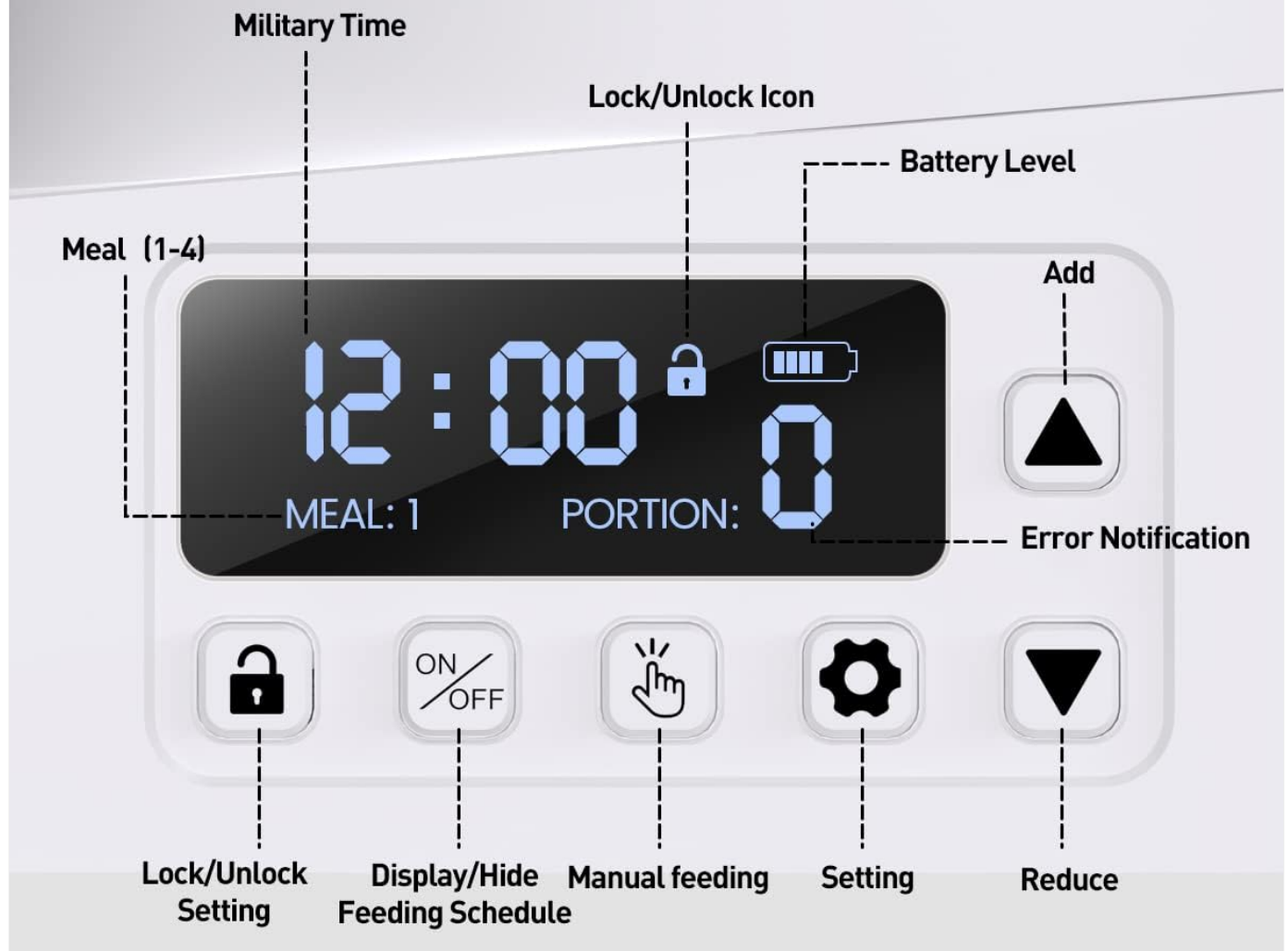
Image 5.1: Control Panel Overview. This image provides a detailed view of the feeder's LED screen and control buttons, with clear labels indicating the function of each icon and button, such as setting, manual feeding, and adjusting meal parameters.
