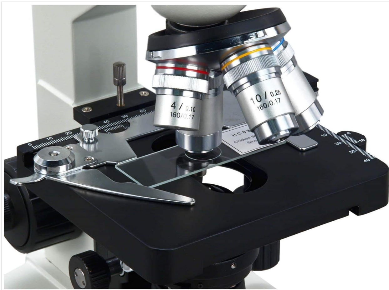
Figure 3: Objective lenses mounted on the revolving nosepiece above the mechanical stage.
