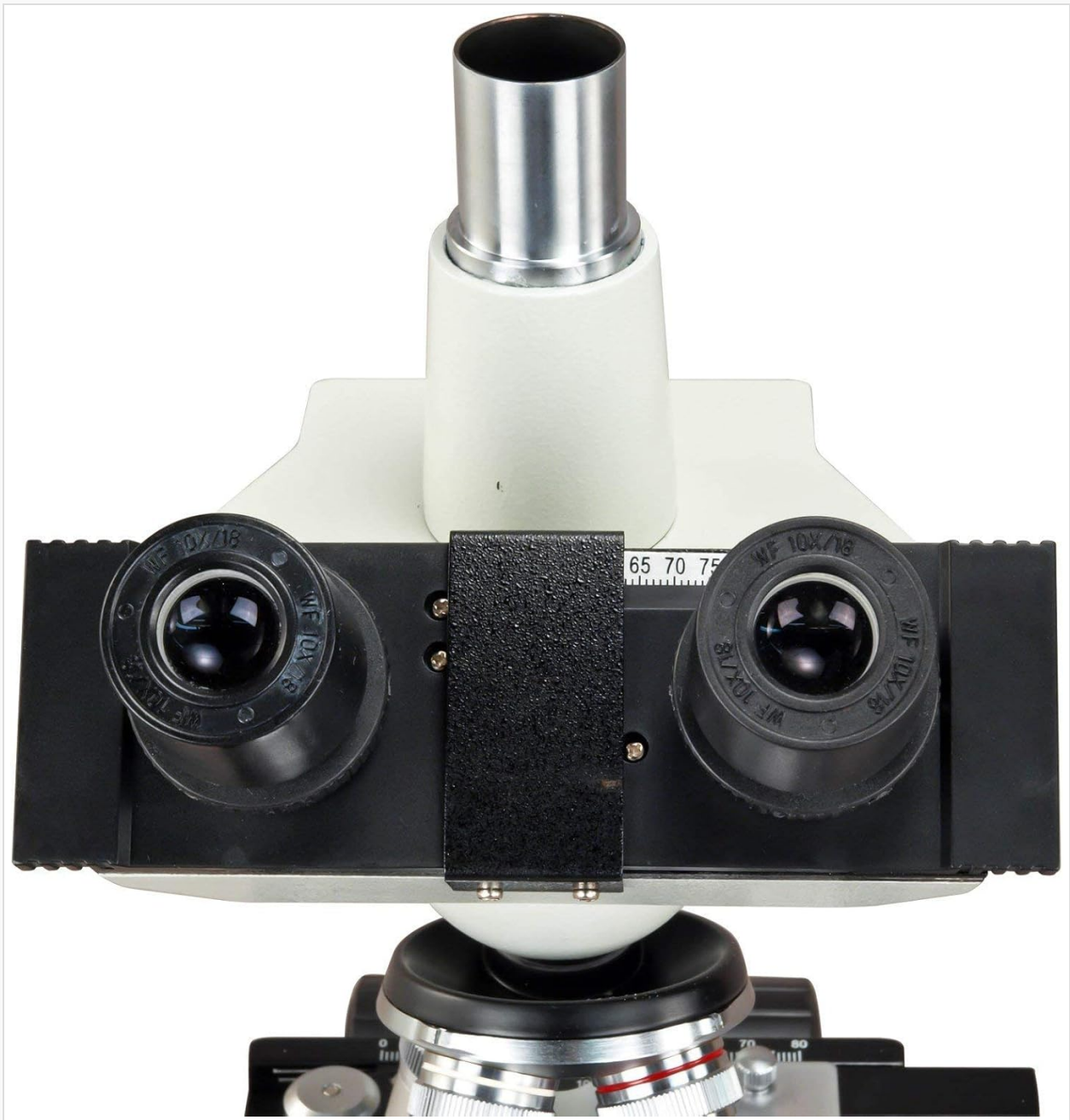
Figure 2: Trinocular head with eyepieces installed.
