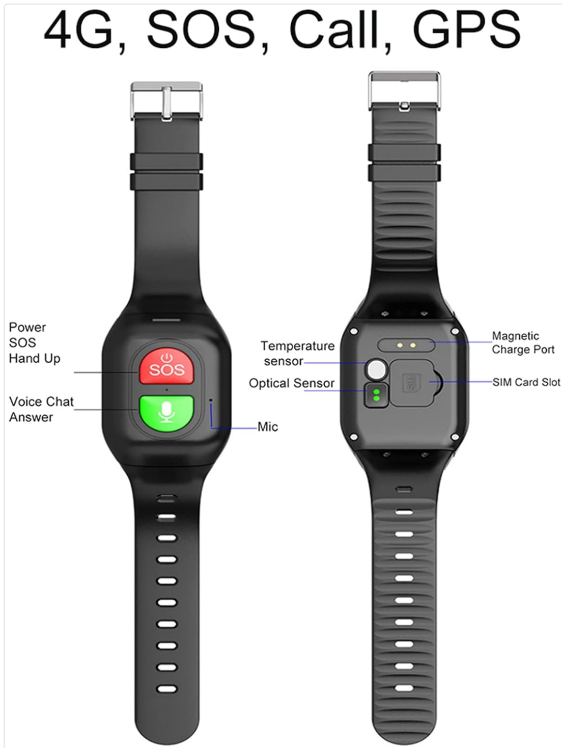
Figure 2.1: Labeled diagram of the smartwatch, highlighting the Power/SOS button, Voice Chat/Answer button, Microphone, Temperature sensor, Optical sensor, SIM Card Slot, and Magnetic Charge Port.
