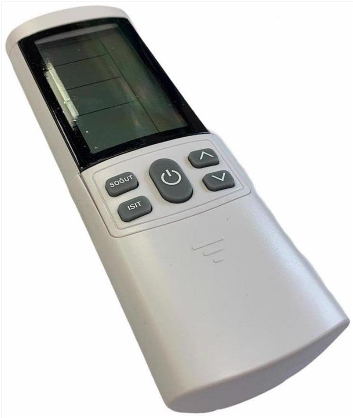
Figure 2.1: Front view of the remote control, highlighting the display and main control buttons.
