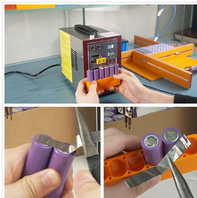
Image: A close-up view showing a nickel strip being welded onto the positive terminal of an 18650 battery.
