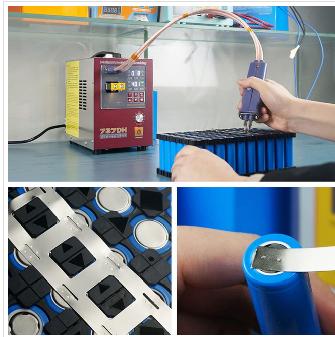
Image: The spot welder being used to attach nickel strips to a series of 18650 batteries, demonstrating the welding process.
