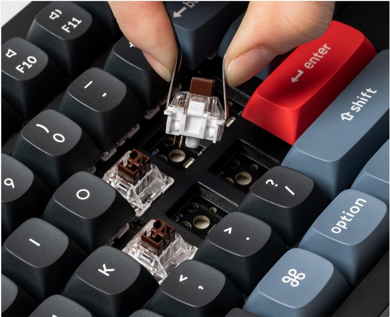
Image 4.2: A hand demonstrating the removal of a mechanical switch from the Keychron V6 keyboard using a switch puller.
