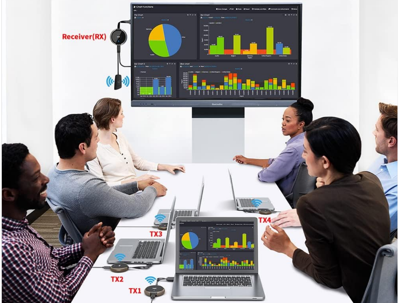
Image: A meeting room setup demonstrating one receiver connected to a display, receiving input from multiple transmitters connected to laptops.
