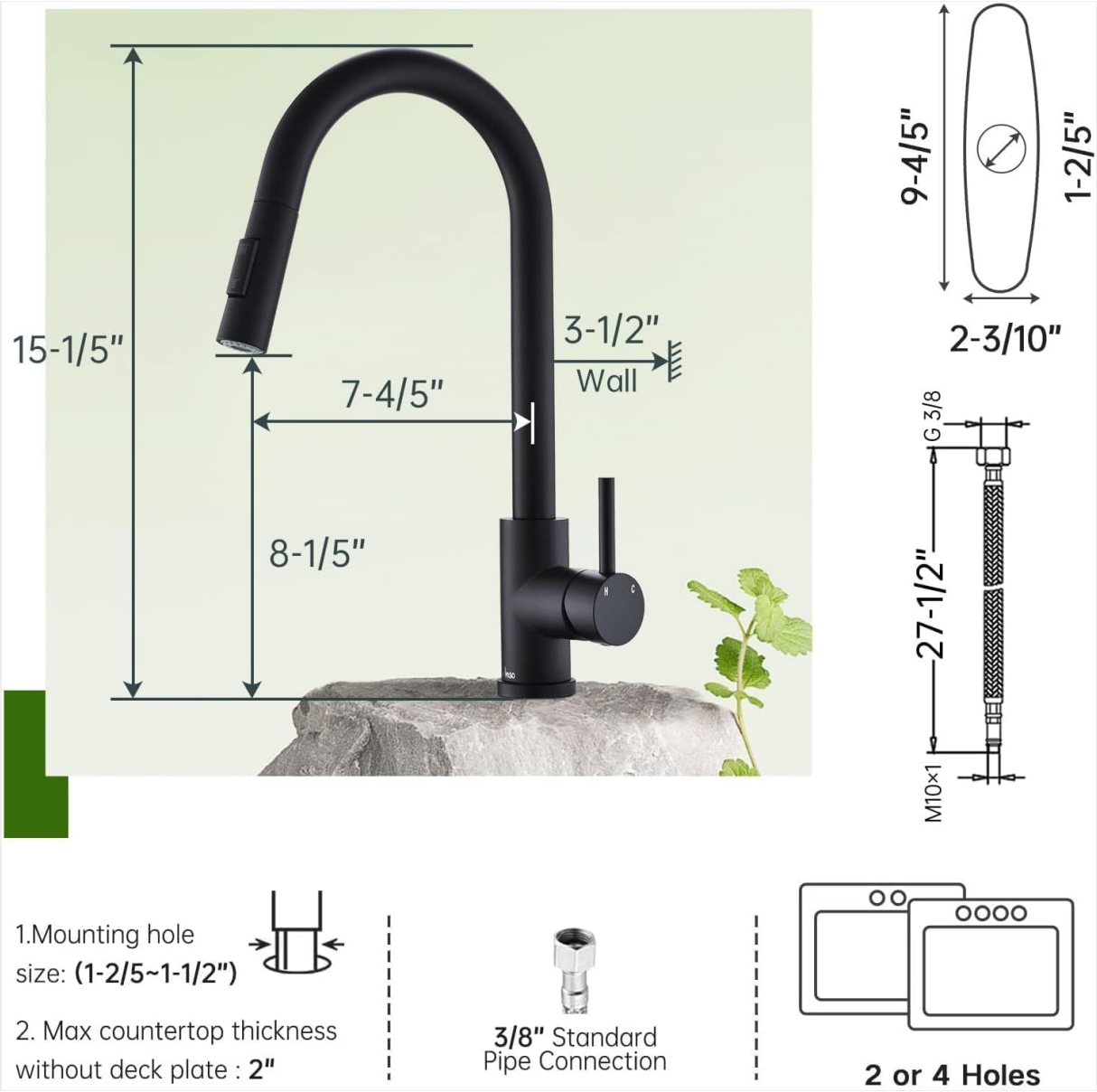
Image: Detailed dimensions and mounting requirements for the APPASO kitchen faucet.
