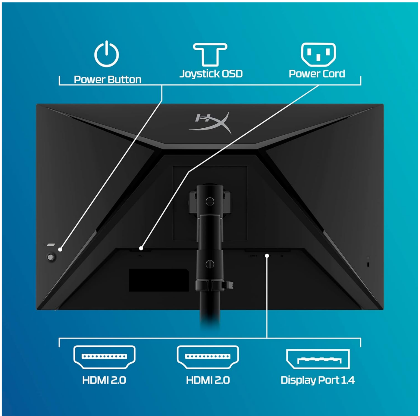
Image: Rear view of the HyperX Armada monitor, detailing the location of the power button, OSD joystick, and input ports (2 HDMI 2.0, 1 DisplayPort 1.4).
