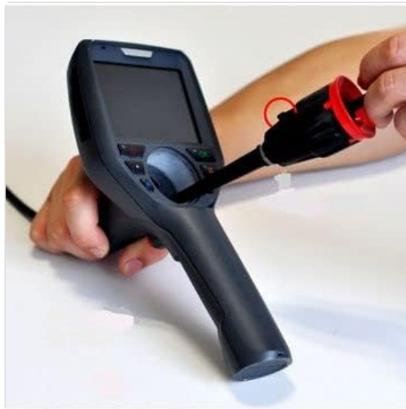
Figure 5: Illustration of connecting the inspection probe to the main unit, ensuring a secure and proper fit.
