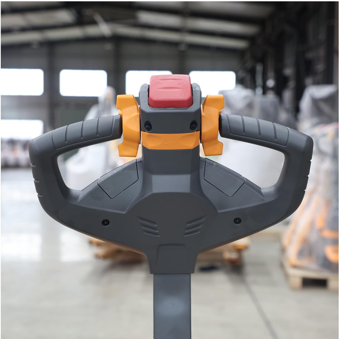
Figure 7: Close-up view of the multi-function control handle with push-buttons and thumb wheels.
