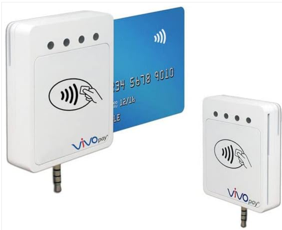
Figure 2: The IDTech VP3300 demonstrating contactless payment functionality and its audio jack connectivity option.
