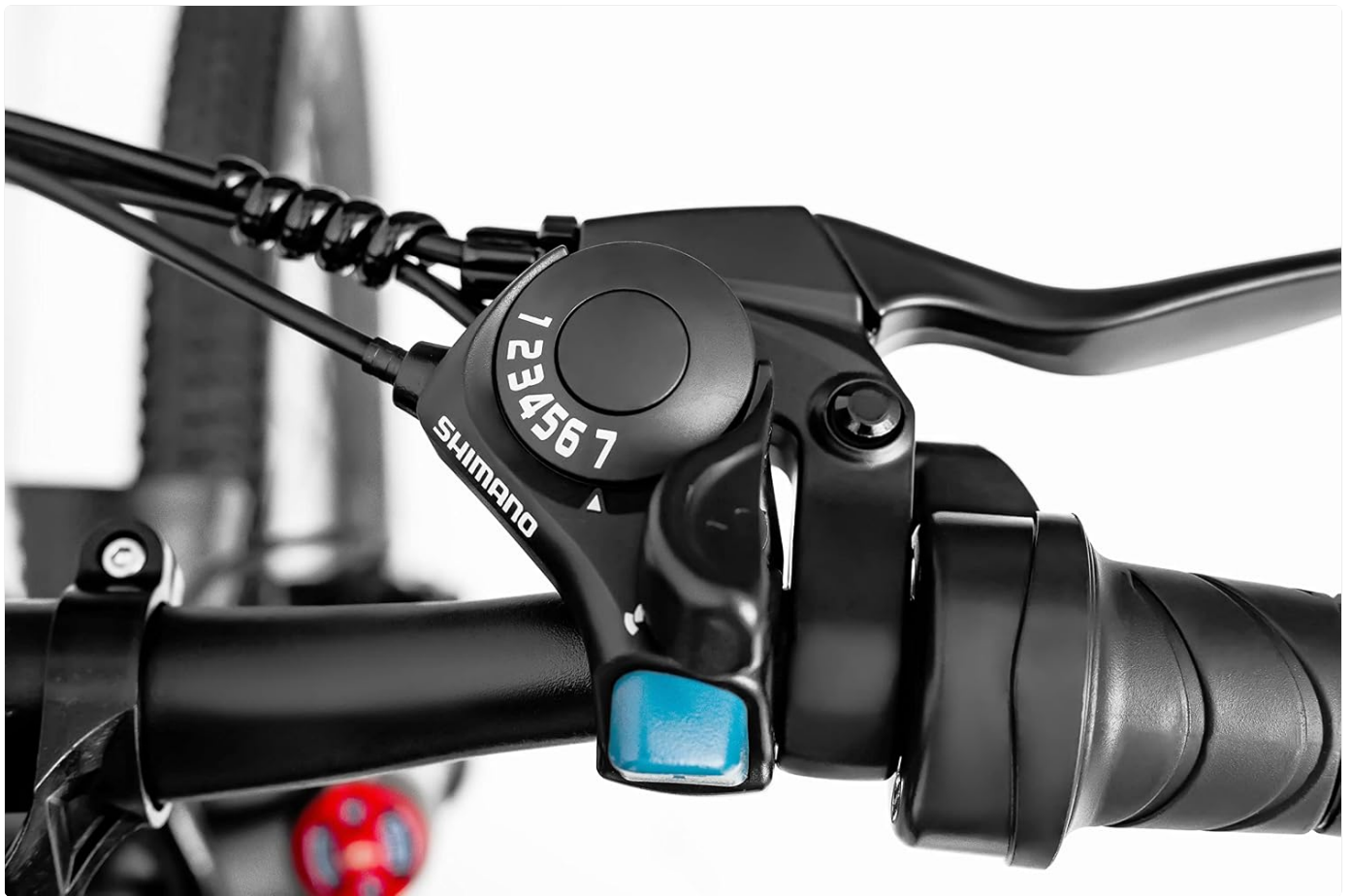
Figure 5: Close-up of the Shimano 7-speed gear shifter and brake lever on the right handlebar. The numbers indicate the selected gear, allowing for precise control over pedaling effort.
