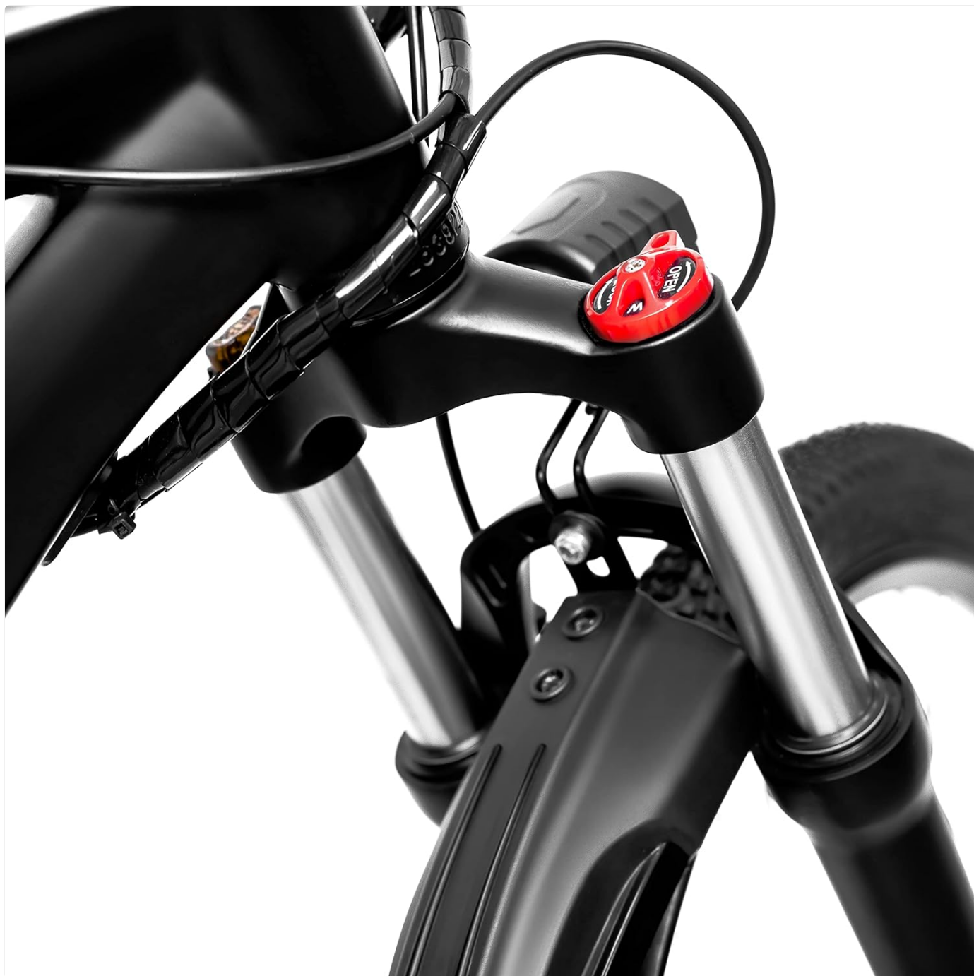
Figure 3: Detail of the front fork suspension adjustment knob. This knob allows riders to fine-tune the suspension's stiffness for different terrains.
