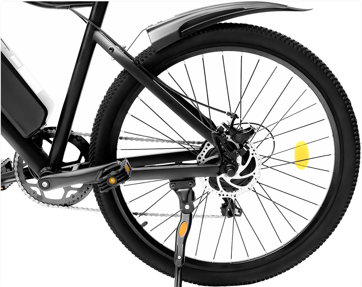
Figure 6: View of the rear wheel assembly, showcasing the disc brake caliper, rotor, and the Shimano derailleur. This area requires regular inspection and maintenance for safe operation.
