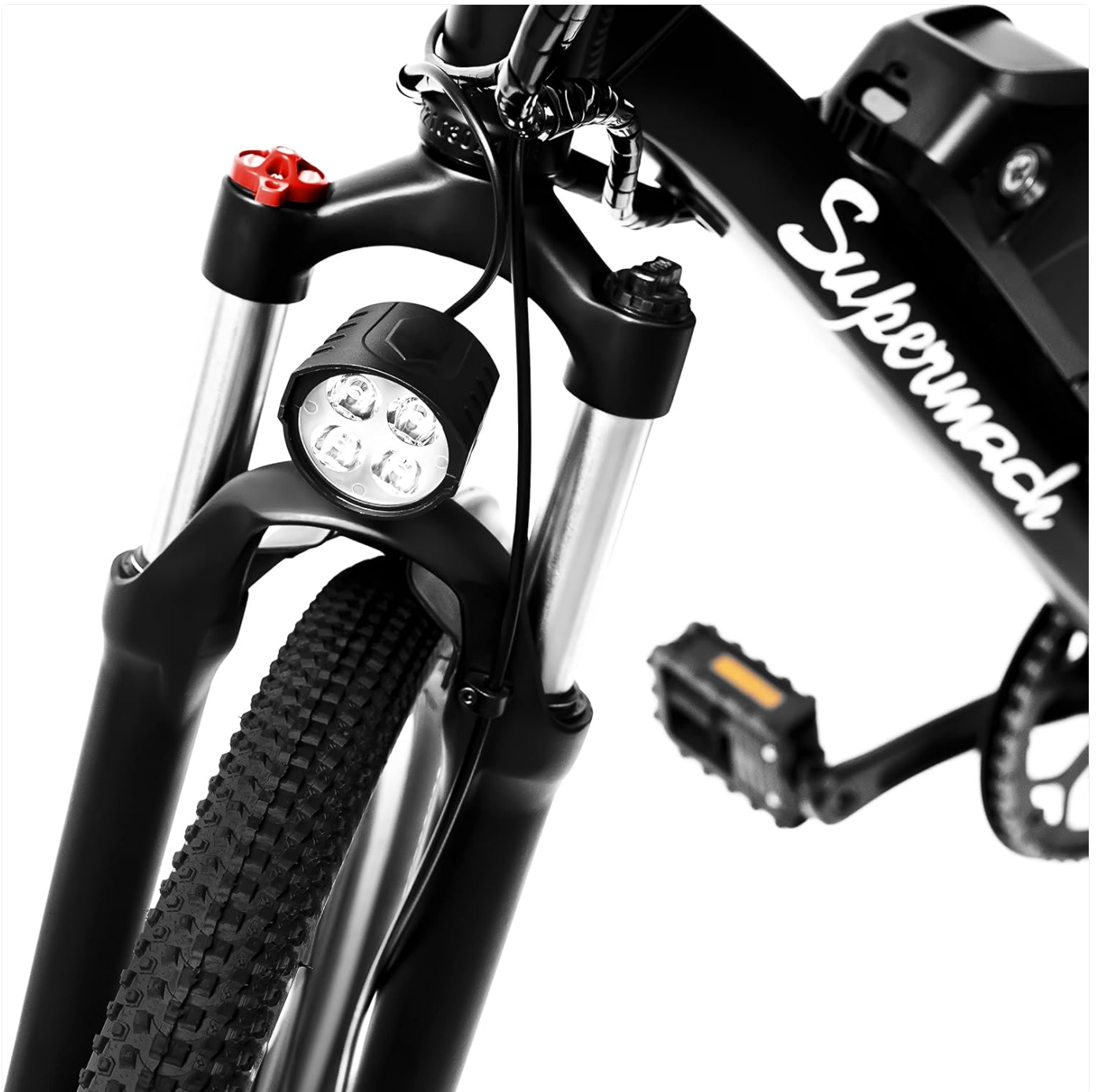
Figure 2: Close-up view of the front headlamp and the front suspension fork. This image helps in identifying the front light for connection and the suspension components for adjustment.
