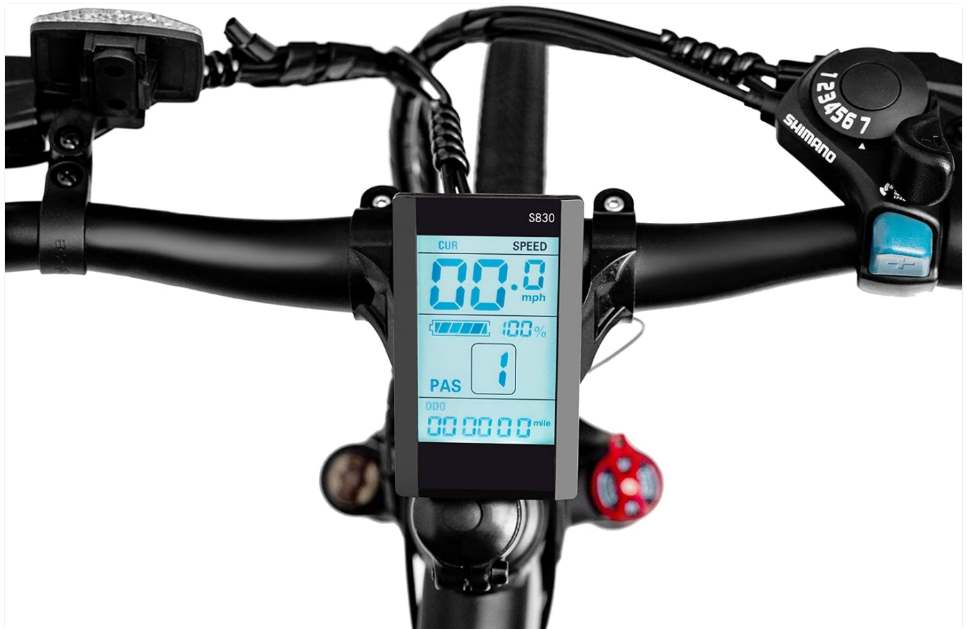
Figure 4: The multifunctional LCD display unit mounted on the handlebars. This display shows current speed (CUR), battery level, pedal assist level (PAS), and total mileage (ODO).
