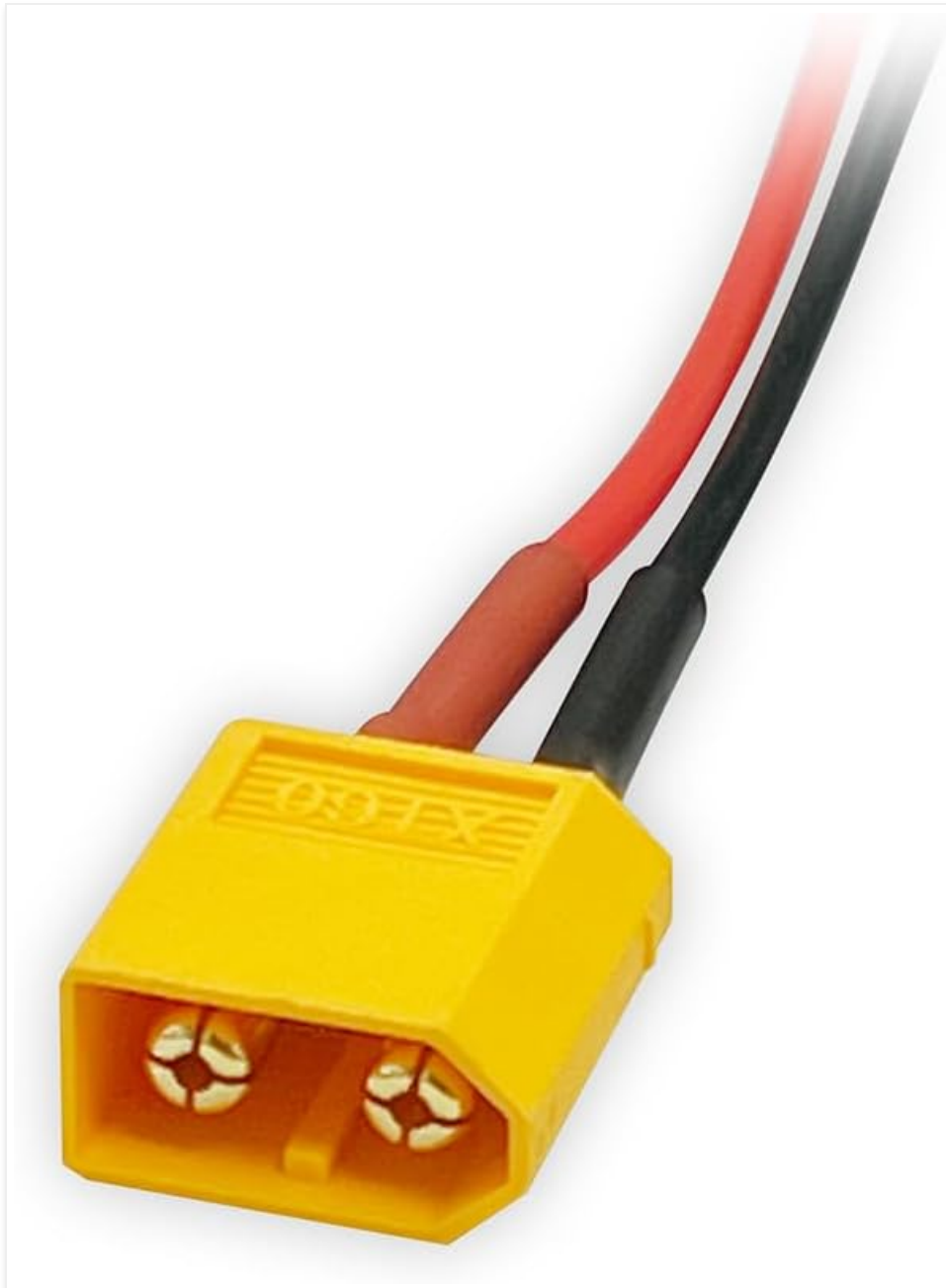
A detailed close-up of the XT60 connector, highlighting its robust design for secure and efficient power connection between the battery and the ESC.
