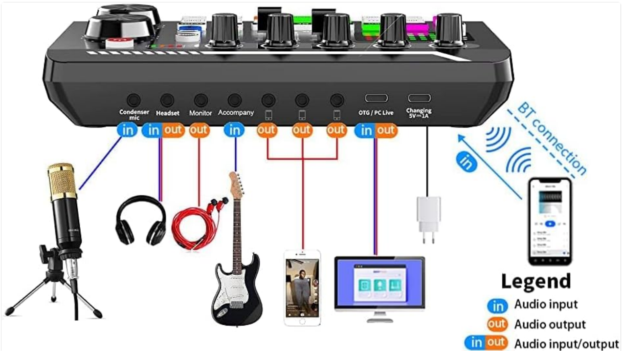
Image 2: Detailed connection diagram for the F998 audio mixer with various devices.
