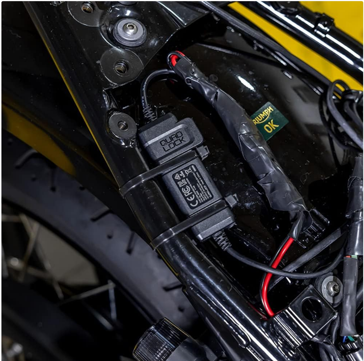
Image: The Smart Adaptor connected to a motorcycle battery using the ring terminal cable.
