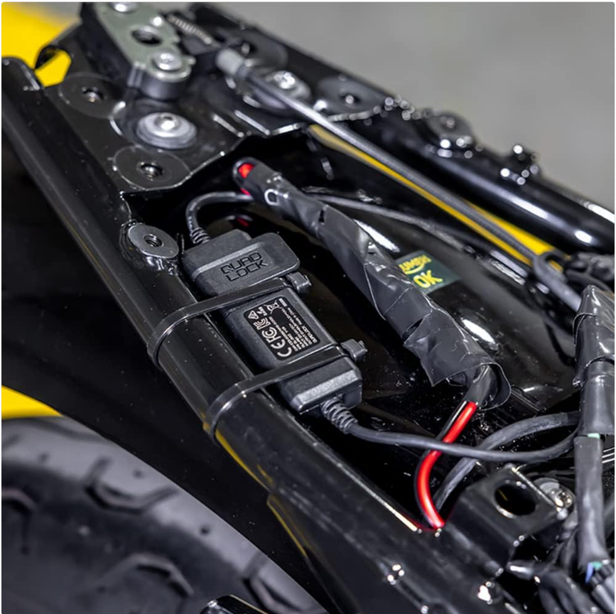
Image: The Smart Adaptor secured to a motorcycle frame using zip ties.
