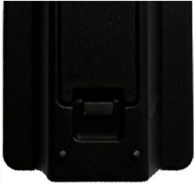
Image 2: Rear view of the remote control, highlighting the battery compartment cover at the bottom.
