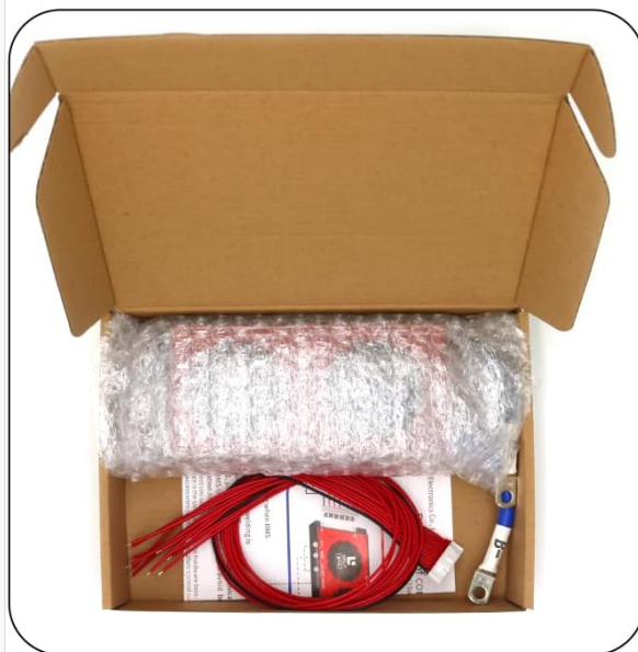
Image: Contents of the DALY BMS package, showing the main BMS unit, the included wiring harness, and a temperature sensor.
