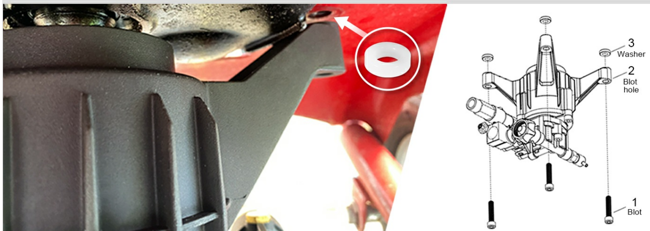
Image: An illustration demonstrating the use of washers to shim the pump for correct alignment with the engine shaft, particularly when the engine shaft length differs.
