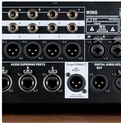
Figure 2: Rear panel highlighting the DC Input and StageConnect power capabilities.
