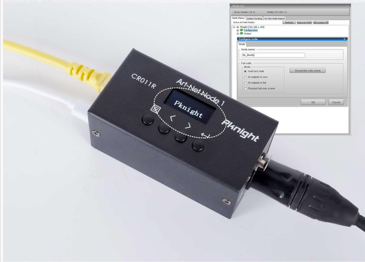
Figure 5: Customizing the device name using DMX Workshop.
