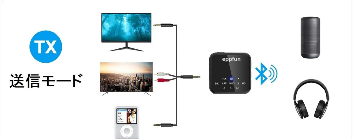
Image 2: TX Mode setup. The diagram illustrates connecting the AK3046C to a TV via AUX/RCA cables and wirelessly streaming audio to two pairs of Bluetooth headphones or a Bluetooth speaker.
