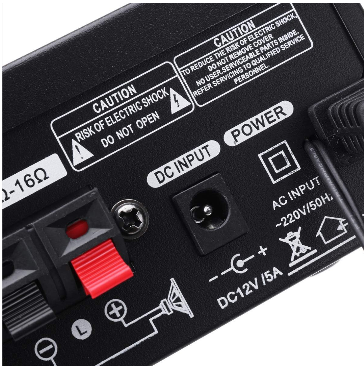
Image: A close-up view of the rear panel's power input section, showing the DC 12V and AC 220V power connections and associated safety labels.
