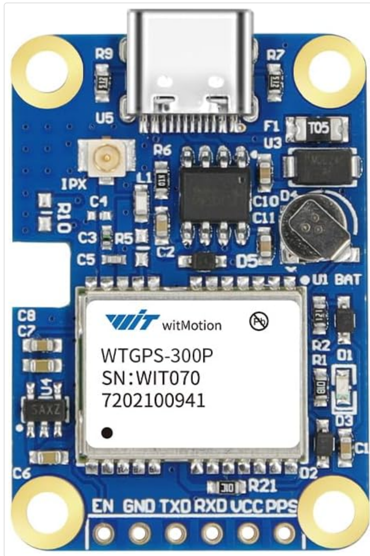
Figure 1: WitMotion WTGPS-300P Module. This image shows the compact design of the module, highlighting the Type-C USB port, IPX antenna connector, and various pins for power and data.
