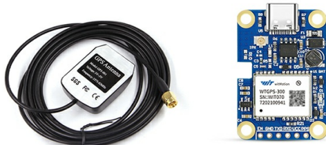
Figure 2: Hardware Analysis of WTGPS-300P. This diagram illustrates key components and interfaces of the module, including the IPX interface for external antennas, Type-C port for PC connection, Farah Capacitance for power backup, GPS-IMU for integrated navigation, and the serial connection points.
