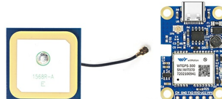
Figure 2: Hardware Analysis of WTGPS-300P. This diagram illustrates key components and interfaces of the module, including the IPX interface for external antennas, Type-C port for PC connection, Farah Capacitance for power backup, GPS-IMU for integrated navigation, and the serial connection points.
