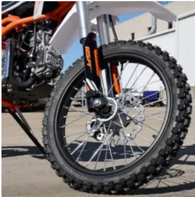
Detail of the hydraulic disc brakes, providing effective stopping power for the dirt bike.
