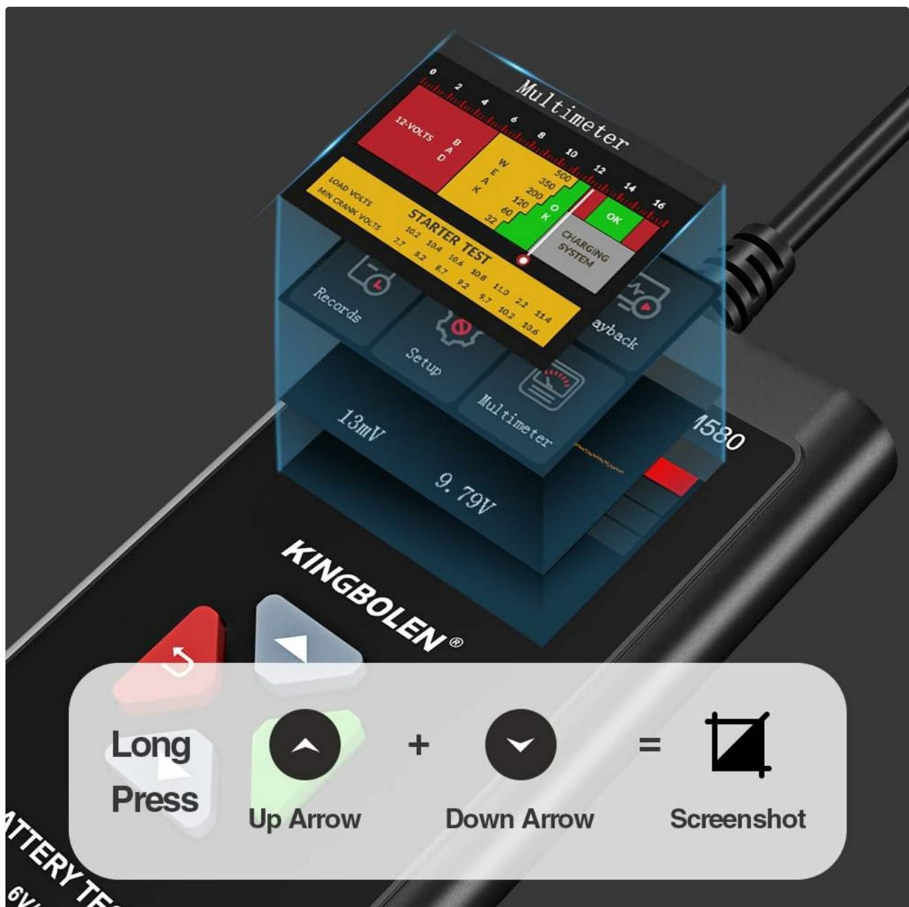
Figure 8: Instructions for using the screenshot function on the BM580.
