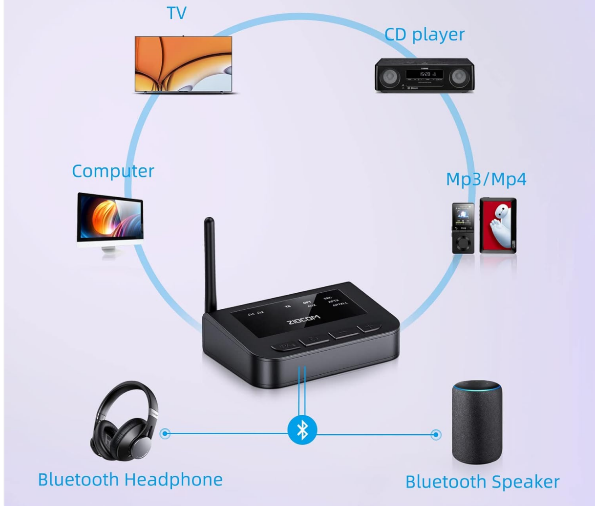
Figure 1: Wide Compatibility of the ZIocom Bluetooth Transmitter. This diagram illustrates how the transmitter can connect to various audio sources (TV, Computer, CD Player, MP3/MP4) and transmit audio to Bluetooth headphones or speakers.
