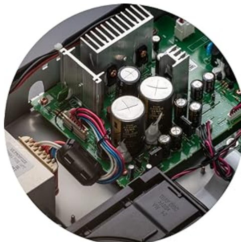
Image 6: Internal view of the Marantz CD 60 power supply section.
