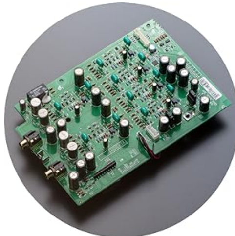
Image 5: Internal view of the Marantz CD 60 circuit board, highlighting the HDAM components.
