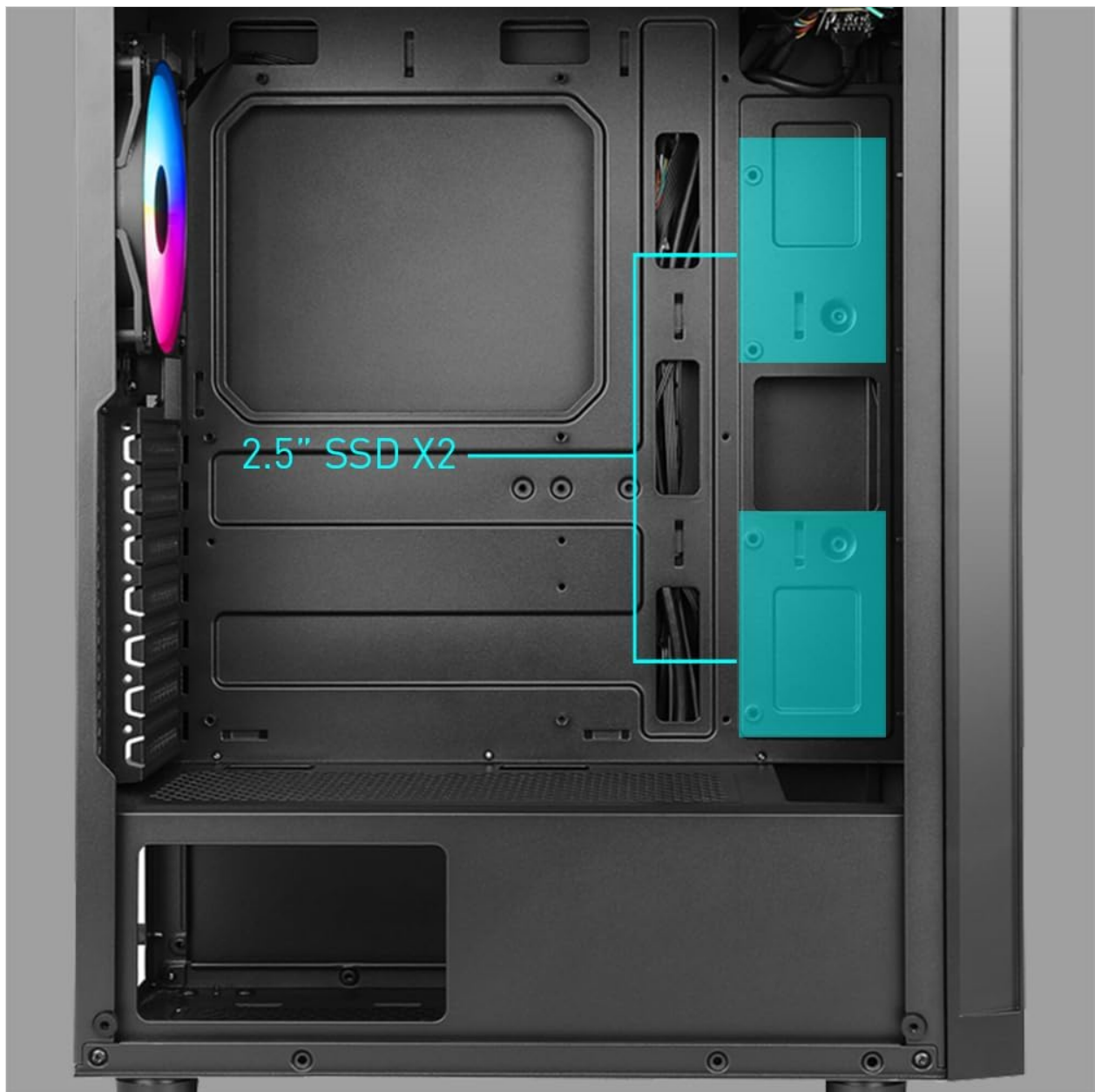
Image 2.3: Internal view showing two dedicated 2.5" SSD mounting brackets located behind the motherboard tray.
