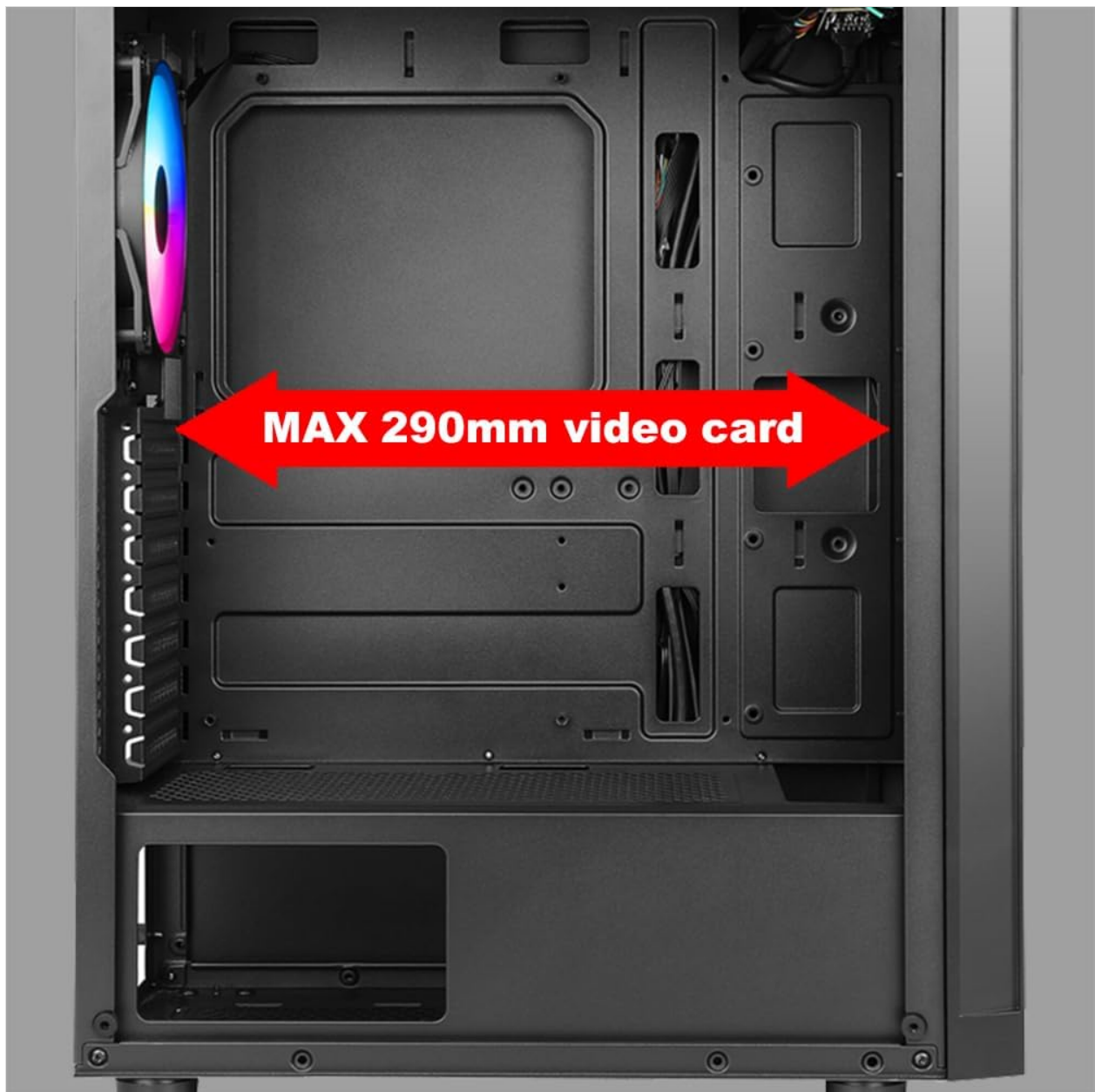
Image 2.4: Internal view illustrating the maximum supported length for a video card, which is 290mm.
