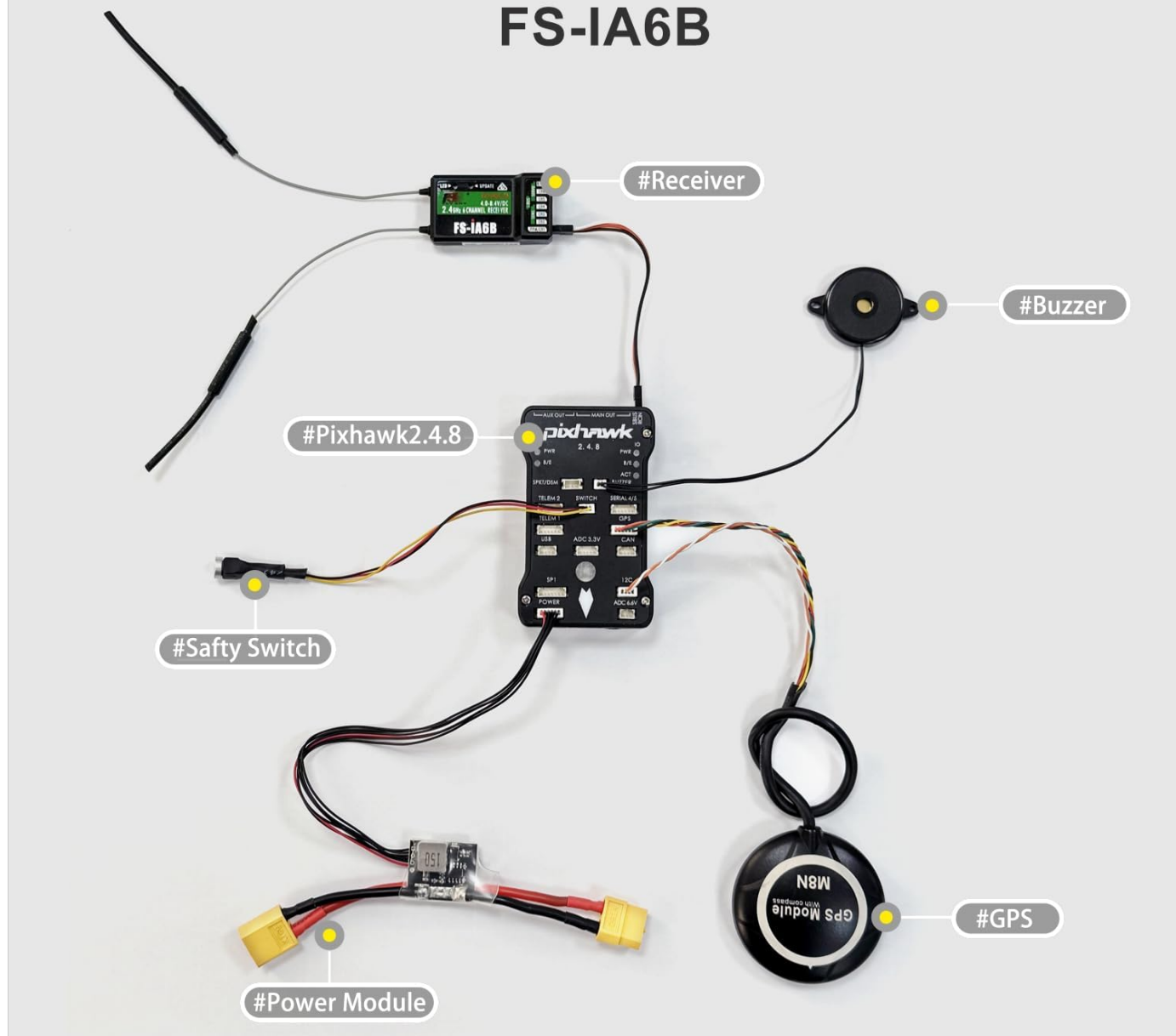
Figure 7: Wiring diagram for FS-IA6B receiver with a Pixhawk flight controller.
