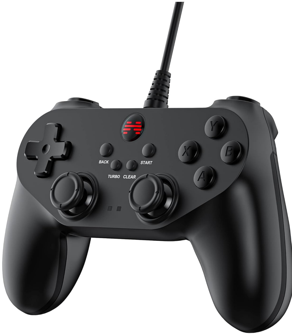
Image: A detailed front view of the BEITONG BAT 2 controller, highlighting the ergonomic design, dual analog sticks, D-pad, action buttons (A, B, X, Y), and central function buttons (Back, Start, Turbo, Clear).
