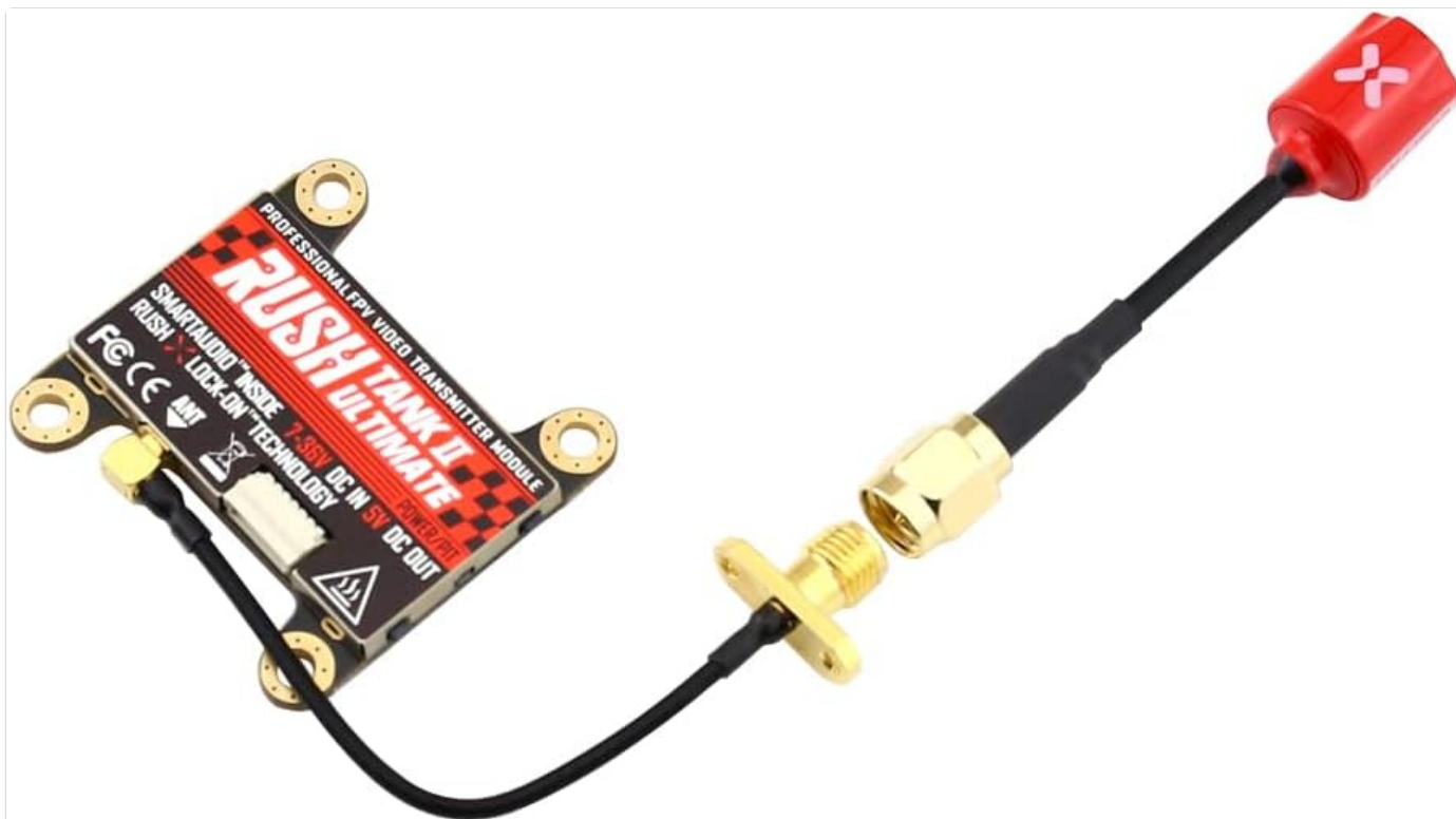
Figure 3.2: Close-up view of the MMCX connector on the VTX and the SMA female connector, illustrating how the adapter cable connects.
