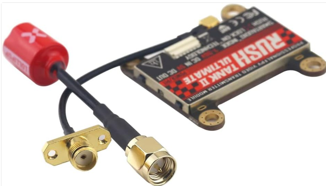
Figure 3.3: The Rush Tank II V2 VTX with the Foxeer Micro Lollipop antenna securely attached, ready for installation.
