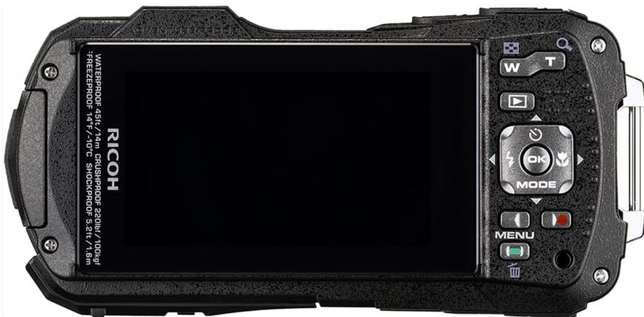
Figure 2: Back view of the Ricoh WG-80 with LCD screen and control layout.
