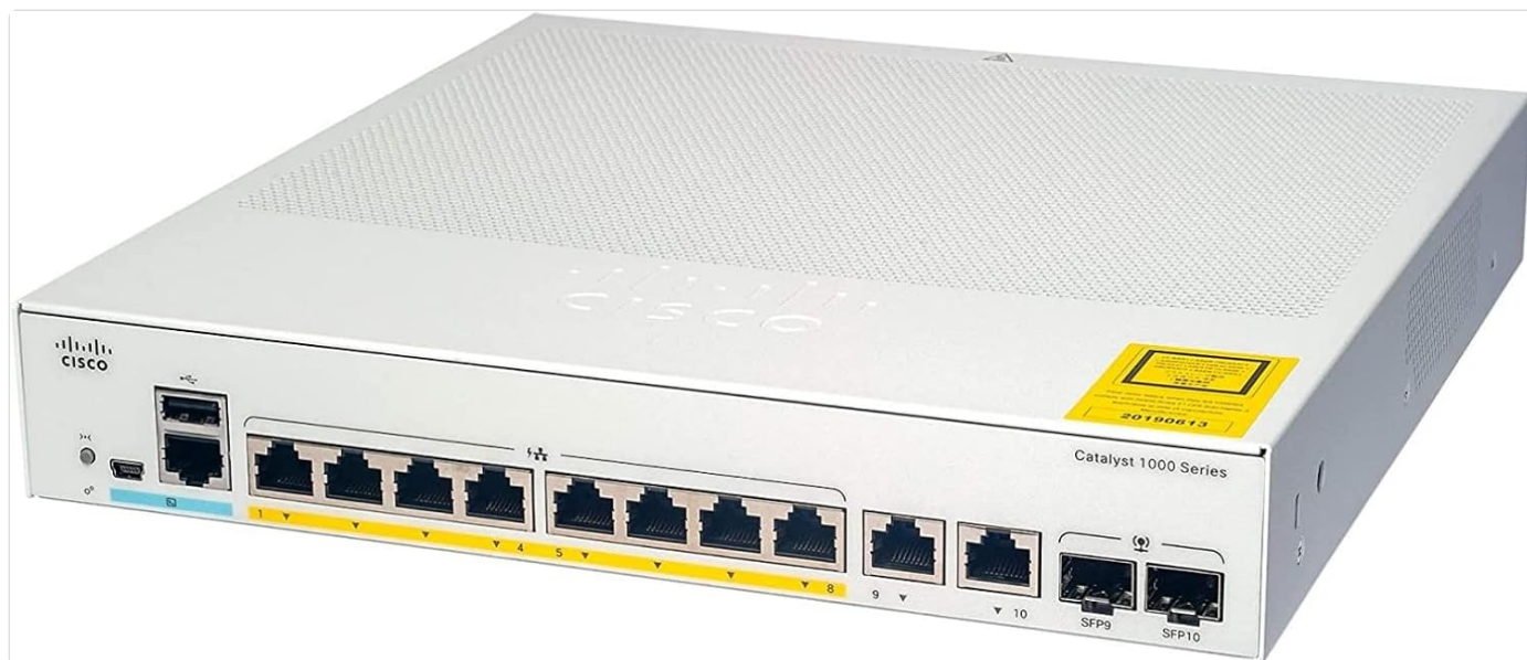
Figure 2.1: Front view of the Cisco Catalyst 1000 Series C1000-8T-2G-L Network Switch, showing the 8 Ethernet ports and 2 SFP/RJ-45 combo ports on the right.
