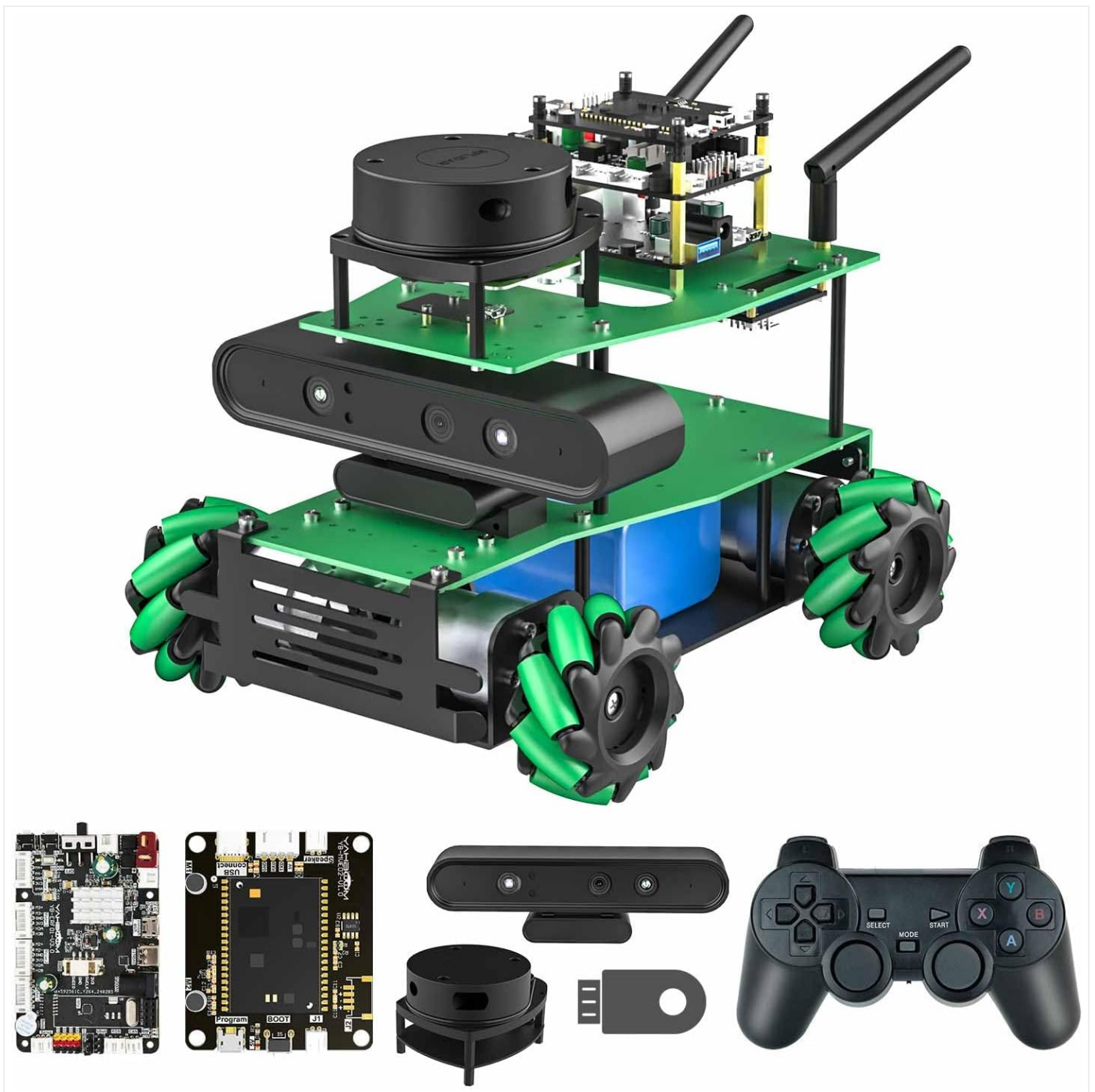
Figure 1: The Yahboom ROS2 Robot Kit, showcasing its main components including the Lidar sensor, depth camera, and Mecanum wheels.
