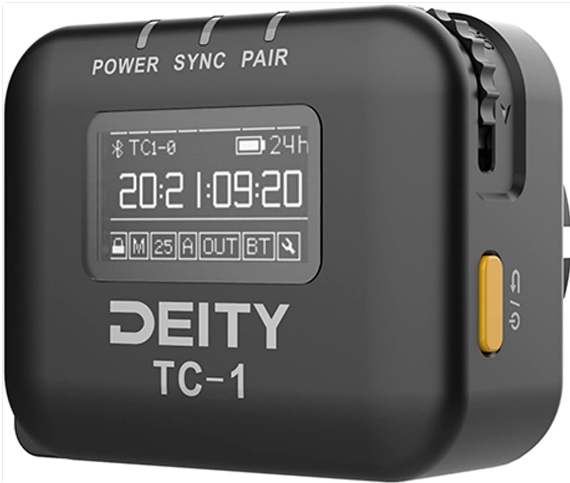
Image: Front view of the Deity TC-1, highlighting its 1-inch OLED display showing timecode, battery status, and connection indicators.
