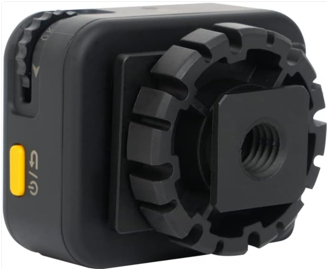
Image: Bottom view of the Deity TC-1, illustrating the attachment point for the removable cold shoe holder.
