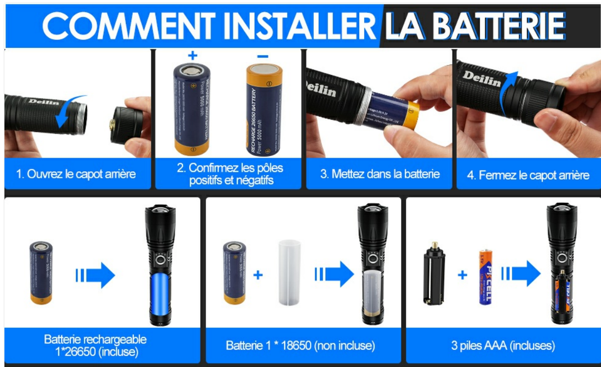
Image: A visual guide demonstrating the steps for installing the battery, including unscrewing the tail cap, inserting the battery with correct polarity, and securing the cap. It also shows options for 26650, 18650 (with adapter), and AAA batteries (with holder).
