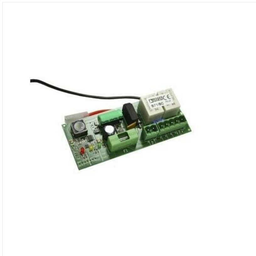
Figure 1: ROGER TECHNOLOGY B71/BC Battery Charger Board. This image displays the compact green circuit board of
