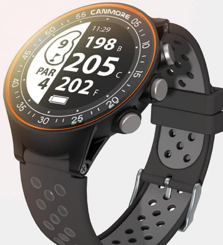
Figure 4.2: Screen indicating shot distance measurement in yards.
