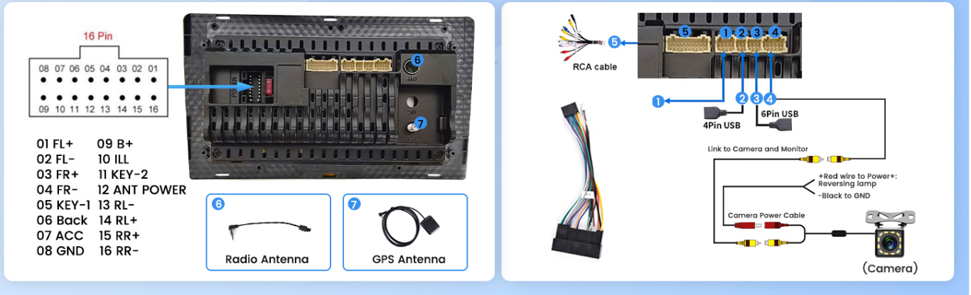
Figure 2: Detailed wiring diagram illustrating connections for the backup camera, USB, and main power harness. Ensure all connections are secure.
