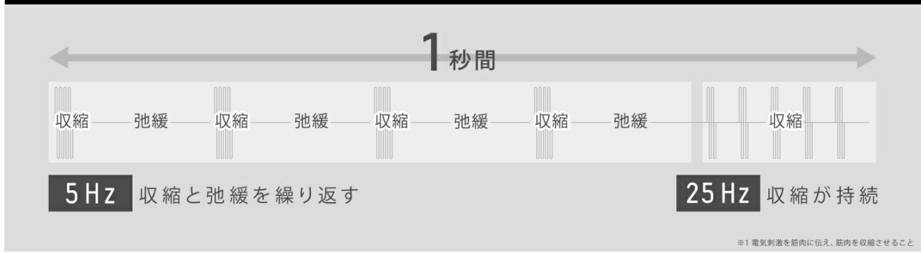
Figure 4: Illustration of the EMS waveform, demonstrating alternating contraction and relaxation at 5Hz and sustained contraction at 25Hz for efficient muscle training.
