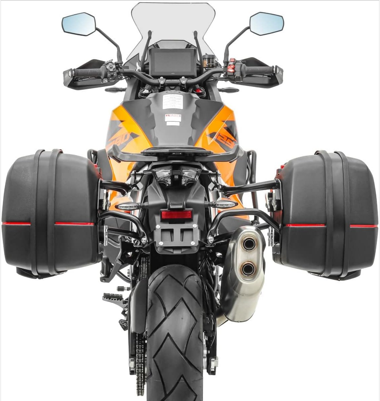
Image 2: Rear view of a motorcycle showcasing both Bagtecs TB8S side cases mounted on a carrier system.
